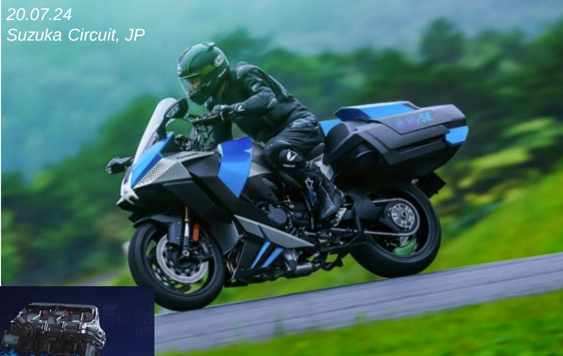
Kawasaki Ninja H2 HySE ICE V4 998 cc, 740 hp 2 liquid H 2 tanks at -253°C
