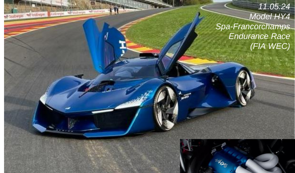
ALPINE Alpenglow – Competition Car - Model HY4: ICE V4 turbo 2000 cc, 340 hp 3 H 2 tanks x 2.1 kg H2 each - Model HY6: ICE V6 biturbo 3500 cc, 740 hp
