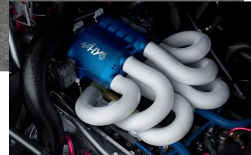
ALPINE Alpenglow – Competition Car - Model HY4: ICE V4 turbo 2000 cc, 340 hp 3 H 2 tanks x 2.1 kg H2 each - Model HY6: ICE V6 biturbo 3500 cc, 740 hp
