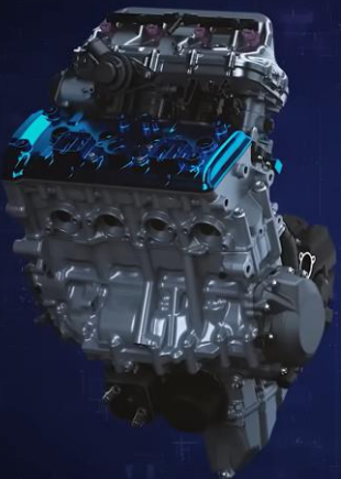
Kawasaki Ninja H2 HySE ICE V4 998 cc, 740 hp 2 liquid H 2 tanks at -253°C
